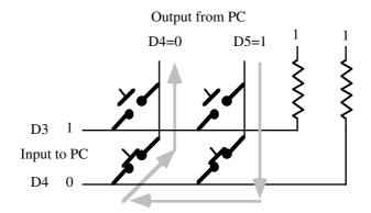
Without a pull up resistor, this dead short could damage the PC's parallel port. By adding two diodes to this circuit, we can protect the PC's parallel port from damage. The revised schematic is
