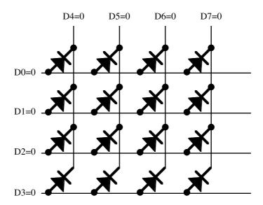
To emit light, an LED requires a logic one on the anode (the rows above) and a logic zero on the cathode (the columns above). Any other combination leaves the LED in the off state. Therefore, all the LEDs in the circuit above will be off. To turn on the LED in the upper left hand corner of this matrix, program D0 with a one and D5, D6, and D7 with a logic one:
