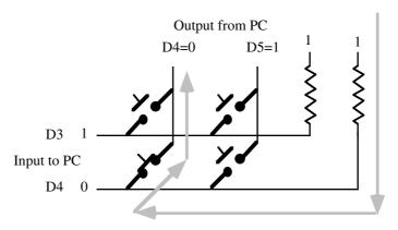
While the D4 column is zero you can read two switches, the two switches connected to the D4 column. Pressing the switches on the other column will not affect the input values. To read the other two switches, you need to program column D4 with a one and column D5 with a zero. Then a zero appearing on the D3 and D4 input lines denote a keypress on the second column of switches.
