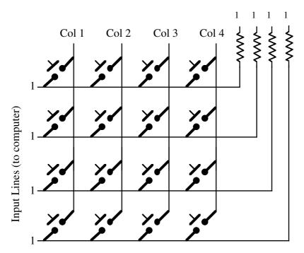
This keyboard matrix requires eight I/O lines, four output lines (Col1..Col4 in this schematic) and four input lines. The combination allows for up to 16 keys, the exact number for a given scanned keyboard is NumInputs \* NumOutputs. To understand how a scanned keyboard works, consider the schematic for the scanned keyboard you will be building for this chapter's laboratory exercises:
