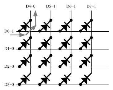
Programming D5, D6, and D7 with a logic one prevents the other three LEDs on the top row from turning on.
