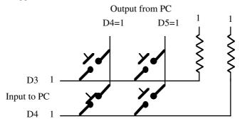
As long as the two columns both contain a one, the inputs on the PC will always be a one even if a switch on the key matrix is in the closed position. This is because the keypress above shorts the D4 column with the D4 row. Since the column and row lines are already one, the value sent to bit four of the input port remains a one.
