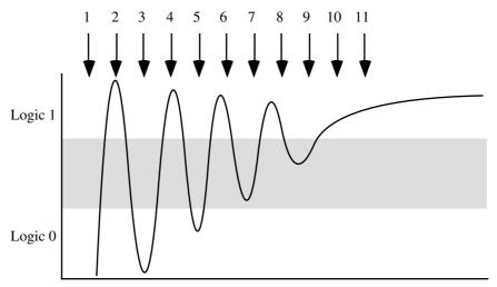
On the first, third, and fifth scans the input is a logic zero (the seventh and ninth readings might also be a logic zero, though these readings are in an indeterminate area). On the second, fourth, sixth, eighth, ten, and beyond readings, the input is a logic one. Therefore, it will appear to the computer that the user has pressed and released the key three times in quick succession. Had this been a computer keyboard, pressing that key once would have produced three keystrokes.
