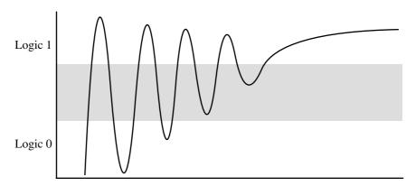
When you first press the switch there is a big burst of current through it. This raises the voltage to a logic one level. The the switch contacts bounce and break the circuit, this cause the voltage to drop back to a logic zero level. The switch contacts bounce several times, repeating this process.
