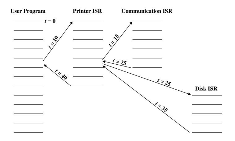
Figure 3.14 Example Time Sequence of Multiple Interrupts [TANE90]
