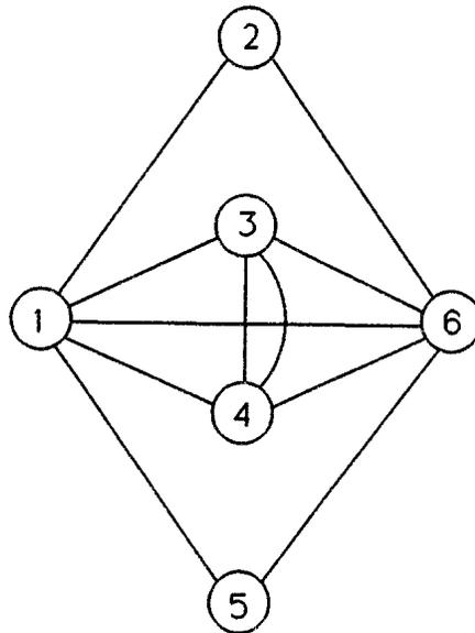
Then by applying the algorithm for finding the Euler tours in  $G^*$ , we have an optimal route  $1 - 2 - 6 - 5 - 1 - 3 - 6 - 4 - 3 - 4 - 1 - 6 - 1$ ,
