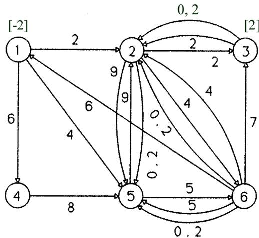
It is now required to find a minimum-cost way of sending 2 flow units from supply vertex 3 to demand vertex 1. By inspection, the minimum-cost path from vertex 3 to vertex 1 is the shortest path  $3 \rightarrow 2 \rightarrow 6 \rightarrow 1$ . Therefore the flow is given by,
