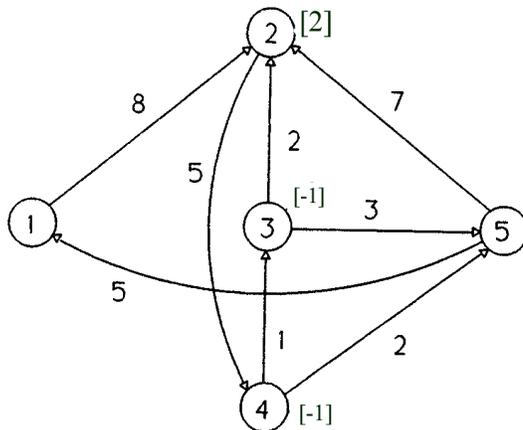
In the network, vertex 2 is a source and vertices 3 and 4 are destinations. The shortest distances  $c(2, 4) = a(2, 4) = 5$  and  $c(2, 3) = a(2, 4) + a(4, 3) = 5 + 1 = 6$ . We have a simple transportation problem:
