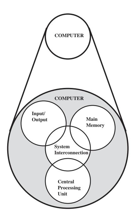
**Figure 1.4 The Computer: Top-Level Structure**
