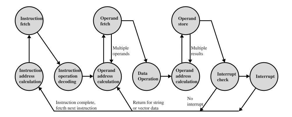
**Figure 3.12** Instruction Cycle State Diagram, With Interrupts
