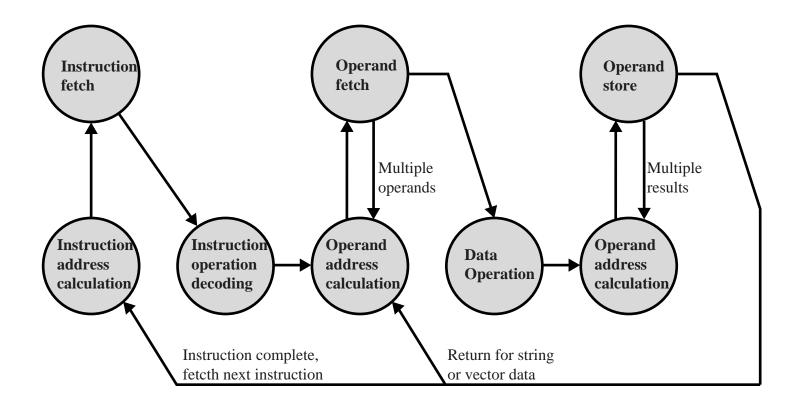
**Figure 3.6 Instruction Cycle State Diagram**
