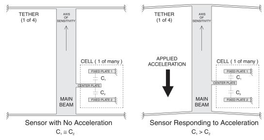
Each of the center plate fits between two adjacent fixed plates, forming a capacitive divider. The two fixed plates are driven with an equal amplitude but opposite polarity square wave signals.
